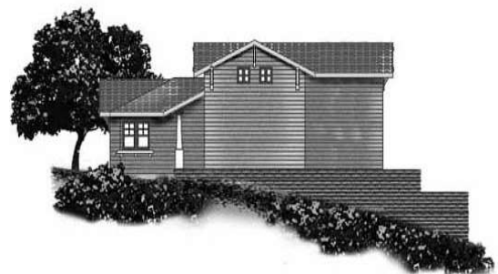
Structure is not suited to the terrain. Extensive grading was used to create building pad, and to terrace site beyond the immediate vicinity of the structure.
