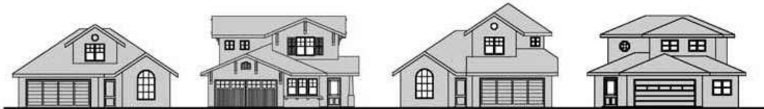
These two-story houses all display roof forms compatible with their architectural style and compatible with neighboring roof forms.
